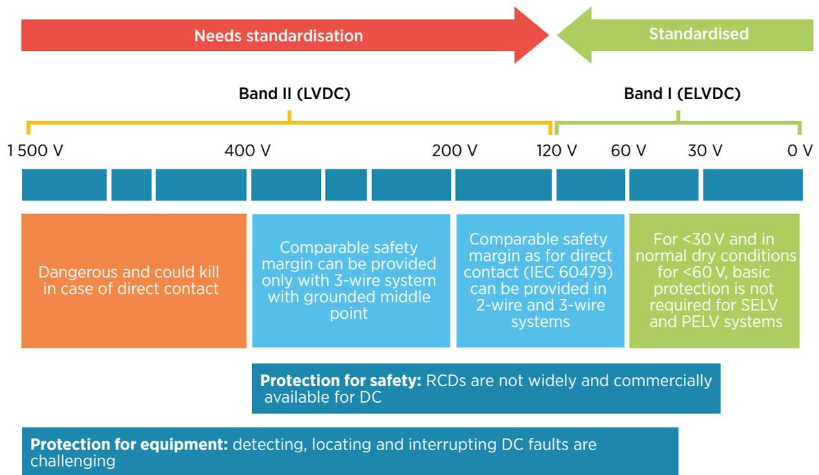
Note: ELVDC = extra-low voltage DC; RCDs = residual-current devices; SELV = separated or safety extra-low voltage; PELV = protected extra-low voltage.
