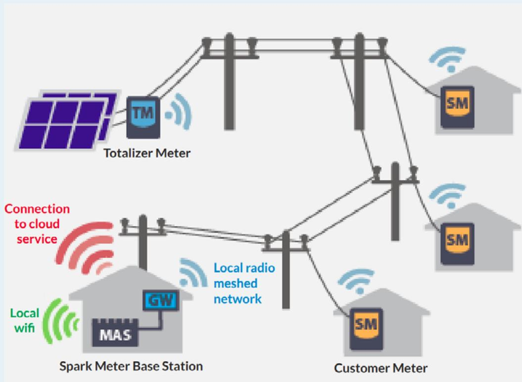
Note: TM = totaliser meter; MAS = SparkMeter base station; SM = customer meter.
