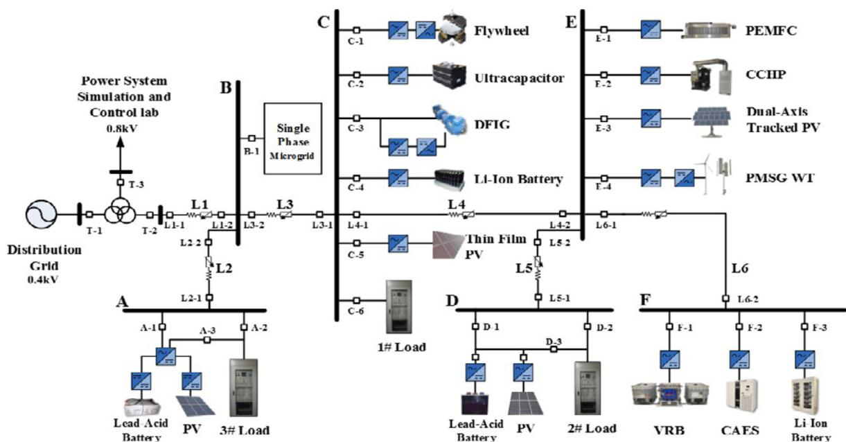
Note: DFIG = doubly fed induction generator; PMSG WT = permanent magnet synchronous generator wind turbine; VRB = vanadium redox battery; CAES = compressed air energy storage.
